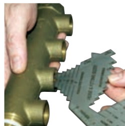
Identify Female Pipe Threads
