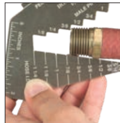
Identify Male Pipe Threads
