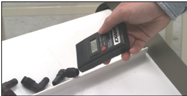
Photo shows how easy it is to use the Static Meter. Just point it at test part. Meter detects both the intensity and polarity of static charges.
