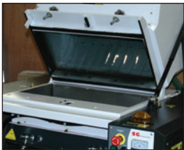
Air spring assisted tilt back adjustable hopper with 3 angle positions makes components accessible for easy cleaning, maintenance and quick blade replacement
