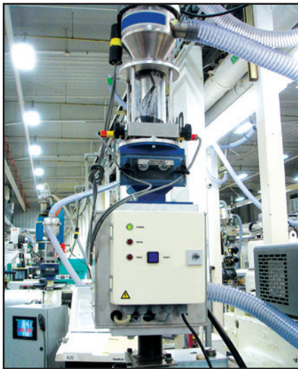
Photo shows Loader, Drawer Magnet and All-Metal Detector
