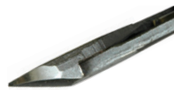
25° blade with slightly rounded back
