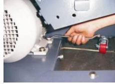
Picture 3-19: Installation of Belt and Belt Pulley 9
