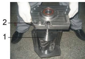
Picture 3-5: Installation of Bearing and Blade Rest 3
