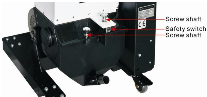
Picture 2-2: Safety System
