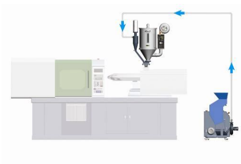
Picture 2-37: Loading With Blower
