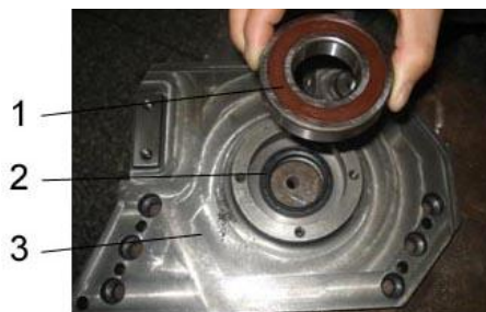
Picture 3-3: Installation of Bearing and Blade Rest 1
