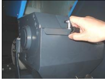
Picture 3-29: Installation of Material Collection Box 4
