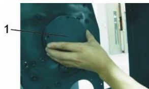
Picture 3-6: Installation of Bearing and Blade Rest 4
