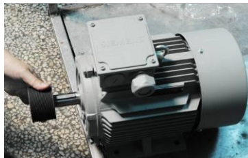
Picture 3-15: Installation of Belt and Belt Pulley 5
