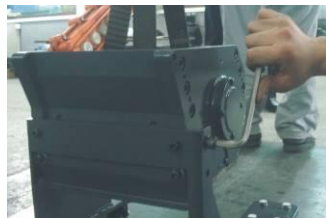
Picture 3-11: Installation of Belt and Belt Pulley 1
