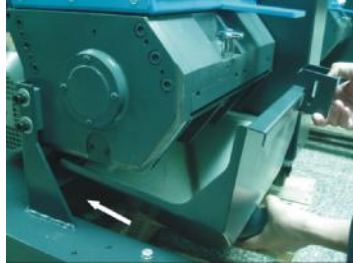
Picture 3-26: Installation of Material Collection Box 1
