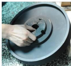
Picture 3-12: Installation of Belt and Belt Pulley 2
