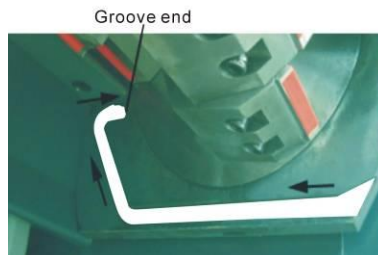
Picture 3-24: Installation of Screen Frame 2
