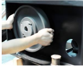
Picture 3-13: Installation of Belt and Belt Pulley 3
