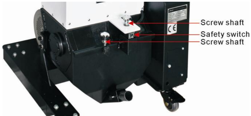
Picture 2-4: Safety System
