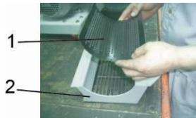
Picture 3-22: Installation of Screen and Screen Frame 1
