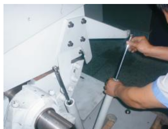
Picture 3-20: Installation of Feed Box and Feed Inletv 4
