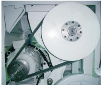
Picture 3-10: Installation of Belt Pulley and Motor 5 (SG-3650)
