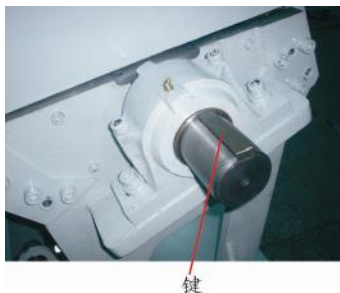
Picture 3-11: Installation of Belt Pulley and Motor 1 (SG-3675)
