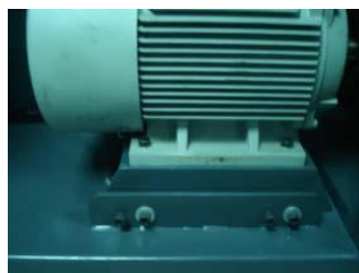
Picture 6-3: Adjustments of V belts
