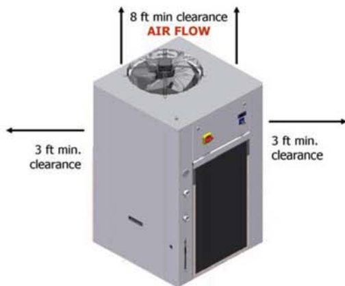
Figure 1. Minimum Installation Clearances
