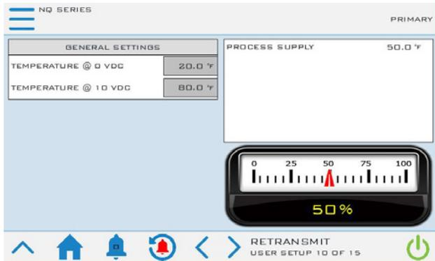
Figure 50 - User Setup – 3-Way Mod Valve Screen
