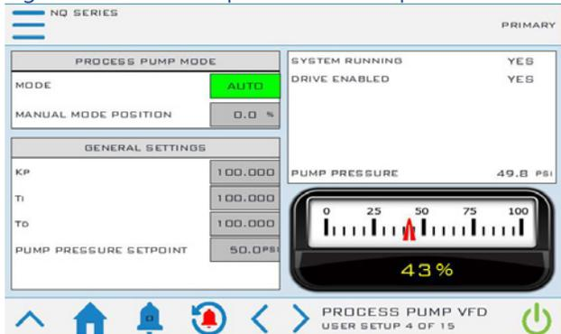
Figure 43 - User Setup – Discharge Control Screen 1
