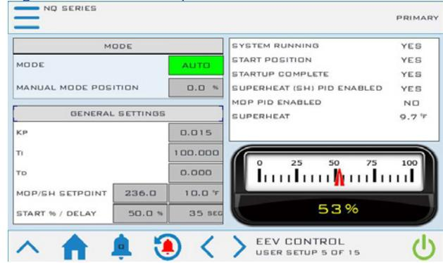
Figure 37 - User Setup – Hot Gas Bypass Screen
