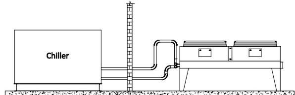
Figure 4 – Condenser Located Above Chiller Unit
