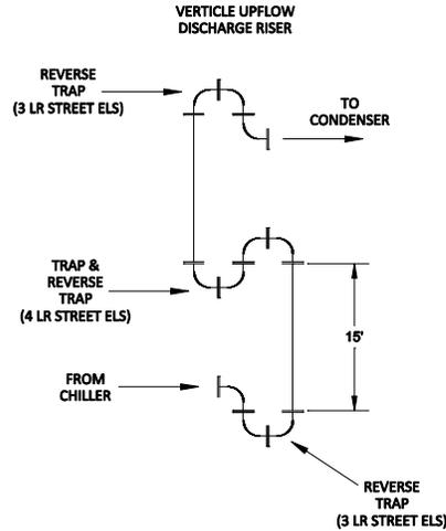
Figure 7 - Double Discharge Riser
