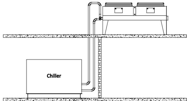
Figure 5 - Condenser Located Below Chiller Unit
