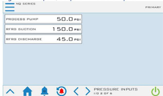
Figure 29 - Inputs/Outputs – Analog Inputs Screen
