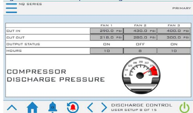
Figure 44 - User Setup – Discharge Control Screen 2
