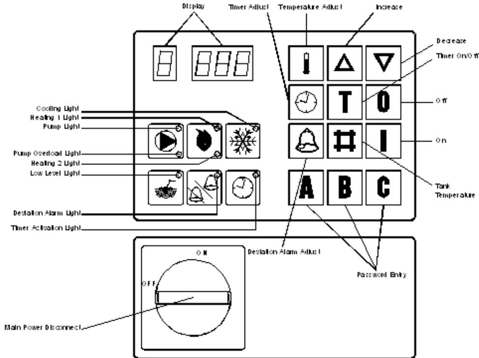
The temperature control unit includes a microprocessor controller designed to perform all control function from the front panel. When a key is depressed, a click will be felt. Unless instructed otherwise, only one key should be pressed at a time.
