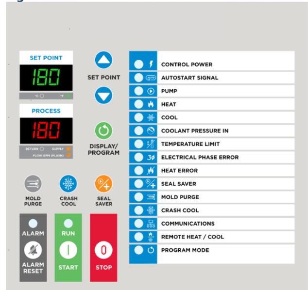
The temperature control unit includes a controller to perform all control functions directly from the front panel. When Control Power is applied, the controller initiates a diagnostic test of each indicating light and display segment which momentarily lights them sequentially. As part of this initial diagnostic test, the program revision level is shown in the temperature display for a moment. After the initial diagnostic sequence is completed, the controller is ready for operation.
